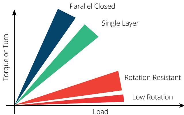
The tendency for any rope to turn will increase as the height of lift increases. In a multi-part reeving system the tendency for the rope to cable will increase as the spacing between the parts of rope decreases. Selection of the correct rope will help to prevent “cabling” and rotation of the load.
