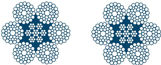
Non Dyform wire rope on adjacent drum laps can cause point contact and accelerated wear.
