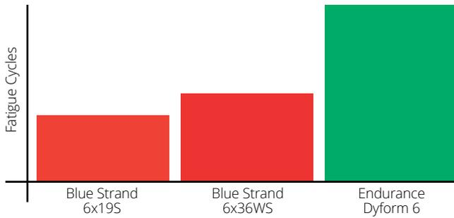
This graph illustrates a “doubling” in life when moving from Blue Strand 6x36 to Endurance Dyform 6. This same relationship can be found when moving from any construction into an equivalent Dyform construction e.g. 18x7 to Endurance Dyform 18 or 35x7 to Endurance Dyform 34LR.
