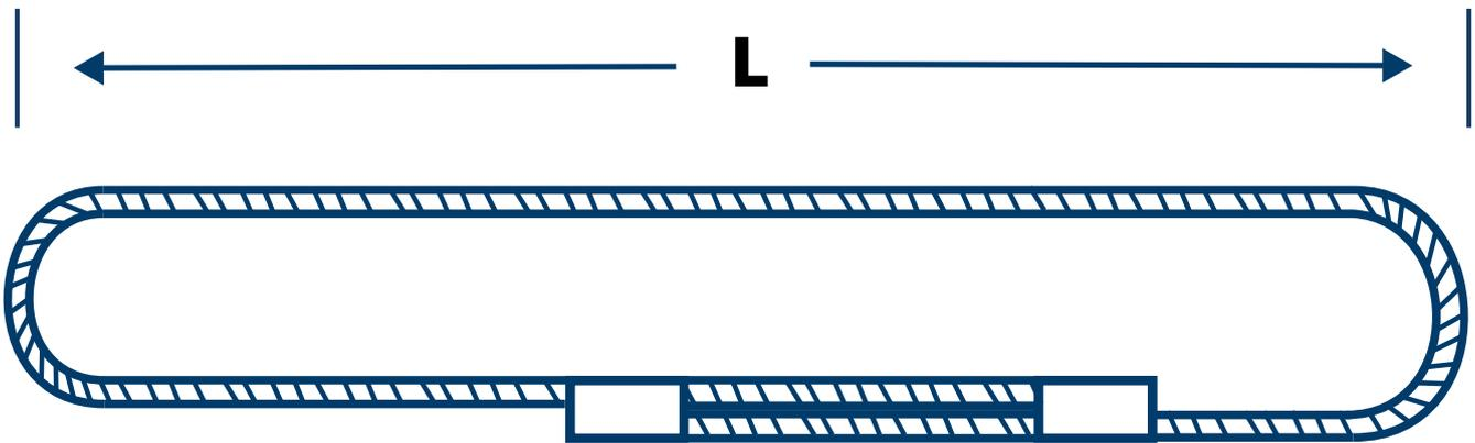
✓ The adjacent ends of the ferrules shall not be less than three times the length of the ferrule apart after pressing.
