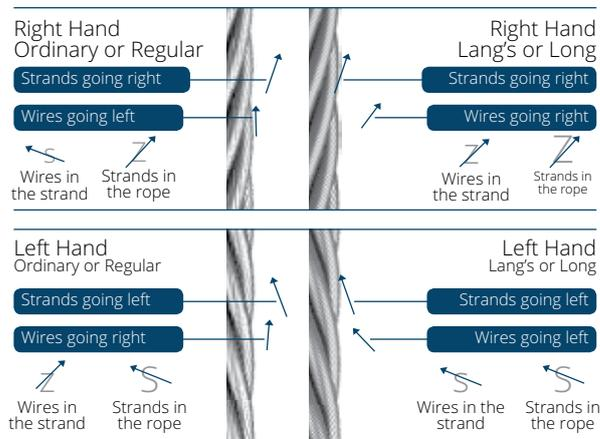
Lang's lay ropes offer greater wear resistance and minimise spooling damage at the cross-over zones when multi-layer wound on winch drum.
