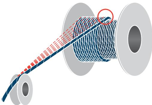
Wire rope on adjacent drum laps can cause point contact and accelerated wear.
